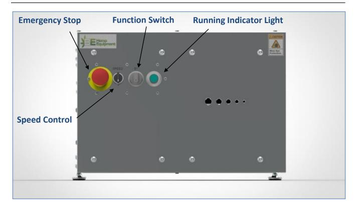
Function Switch: Able to control operation between OFF, ON, AND REVERSE function
