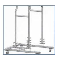
d. Assemble Bracket (item b) onto Frame Assembly using M8 x 40mm screws, M8 washers, and M8 Nuts.
