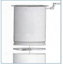
c. Remove screw on outlet of Cyclonic Funnel Assy and place to the side. Install hose and use hose clamp to secure hose to Cyclonic Funnel.
